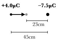
The change in potential energy is  $\Delta PE = PE_f - PE_i$ . The initial potential energy of this configuration is
