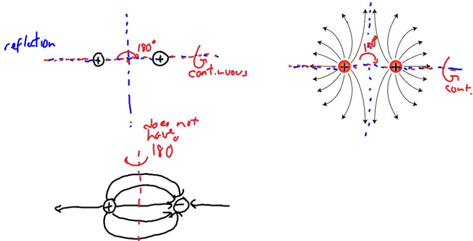
We can use Symmetry & Gauss' Law to find the electric field of
