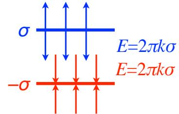
(b) Call the bottom plate  $y = 0$  and the top plate  $y = d$ , so that up is the positive  $+y$  direction. The electric field is constant, and  $E_y = -4\pi k\sigma$ . The potential difference is
