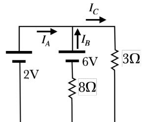
$$+2 - 6 + 8I_B = 0 \quad \text{or} \quad -2 + 6 - 8I_B = 0$$
