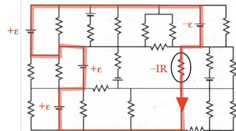
There is a simple loop through the resistor which only includes that one resistor. Going clockwise around this loop gives us  $+12 + 12 + 12 - 12 - 4I = 0 \Rightarrow 24 = 4I \Rightarrow I = 6\text{ A}$
