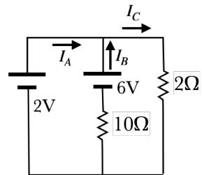
$$+2 - 6 + 10I_B = 0 \quad \text{or} \quad -2 + 6 - 10I_B = 0$$
