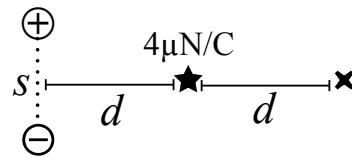
**3** (b) D What is the magnitude of the electric field  $2d$  from the dipole (at the X)?
