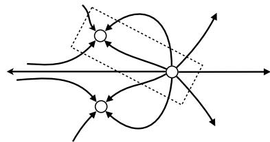
9. **D** Consider two charges: a  $-2\ \mu\text{C}$  charge on the left, and  $+1\ \mu\text{C}$  charge on the right. Which of the following shows the correct electric field lines of these two charges?
