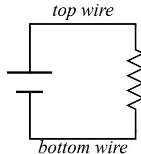
18. In this circuit, the current through the battery is 2 A.
