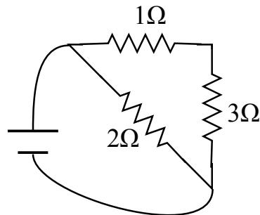
3 (b) Find the effective resistance of all three resistors via resistance reduction.
