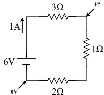
(c) If the potential at the lower-left corner of the circuit is 0 V, what is the potential  $V$  at the upper-right corner of the circuit?
