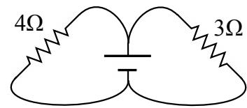
$$G_{\text{eff}} = \frac{1}{4} + \frac{1}{3} = 0.583 \text{ S} \implies R_{\text{eff}} = \frac{1}{G_{\text{eff}}} = 1.7 \Omega$$
